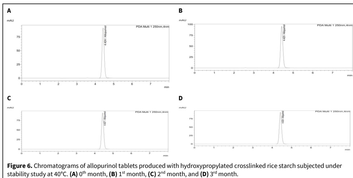
**Figure 6.** Chromatograms of allopurinol tablets produced with hydroxypropylated crosslinked rice starch subjected under stability study at 40°C. (A) 0<sup>th</sup> month, (B) 1<sup>st</sup> month, (C) 2<sup>nd</sup> month, and (D) 3<sup>rd</sup> month.
