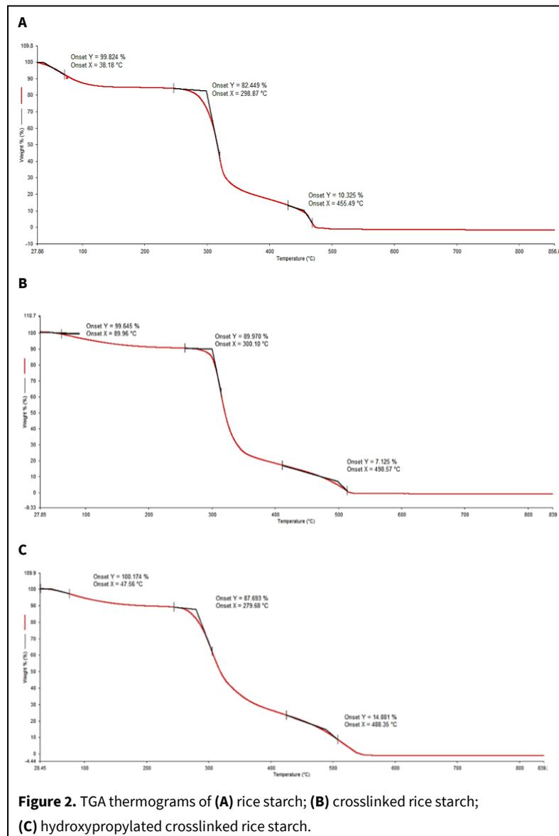
**Table 3.** TGA thermograms of rice starch, crosslinked rice starch, and hydroxypropylated and crosslinked rice starch.
