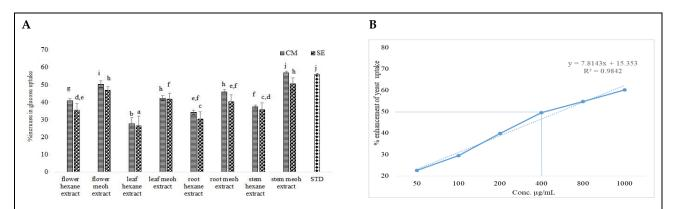
**Figure 2. (A)** Extraction mode impact on increasing glucose uptake by different extracts and the standard; **(B)** the  $EC_{50}$  of stem methanol extract indicated at 400 µg/mL.
