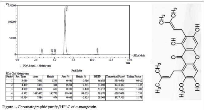
Chromatogram exhibits the peak of  $\alpha$ -mangostin detected at the retention time of 6.372 min with a quantity area of 98.434%. The right side shows the structure of the  $\alpha$ -mangostin compound.
